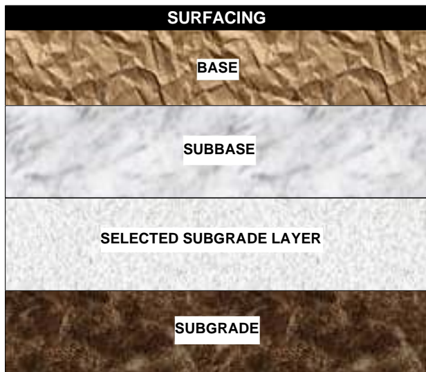
Figure 2.76: Typical Pavement Layers in Flexible Pavements
