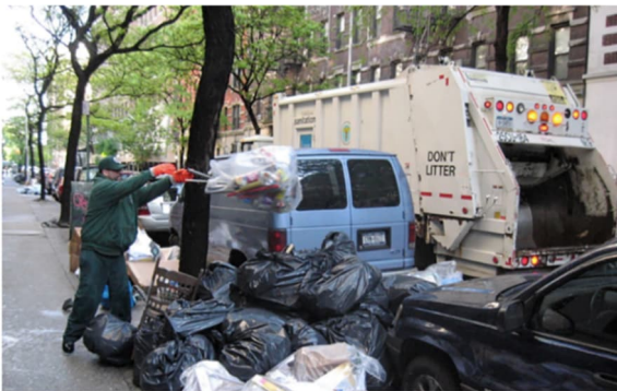
Example of a rear load compactor truck for door-to-door waste collection
