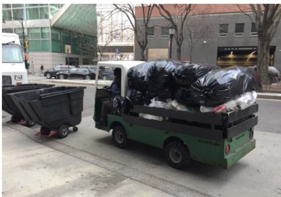
Example of a smaller vehicle used to collect and transport waste from centrally located waste bins & skips.
